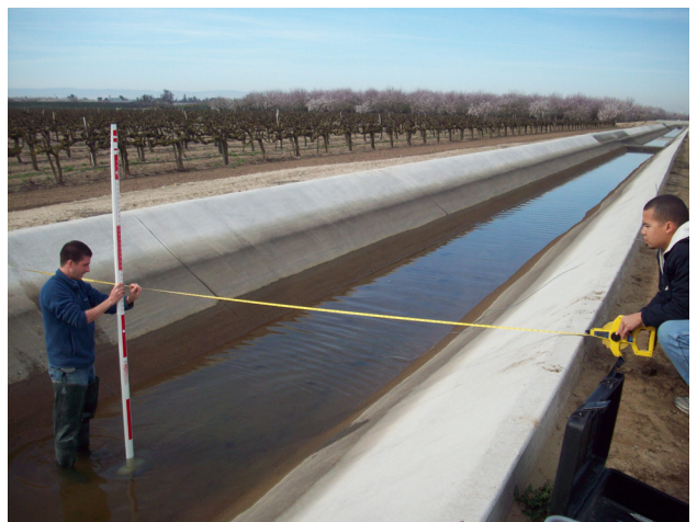
While Doppler flow meters can be highly accurate, user setup and attention to detail can make the difference between good and bad flow data. Of particular importance is verification of the cross section dimensions at the location where the sensor will be installed.
