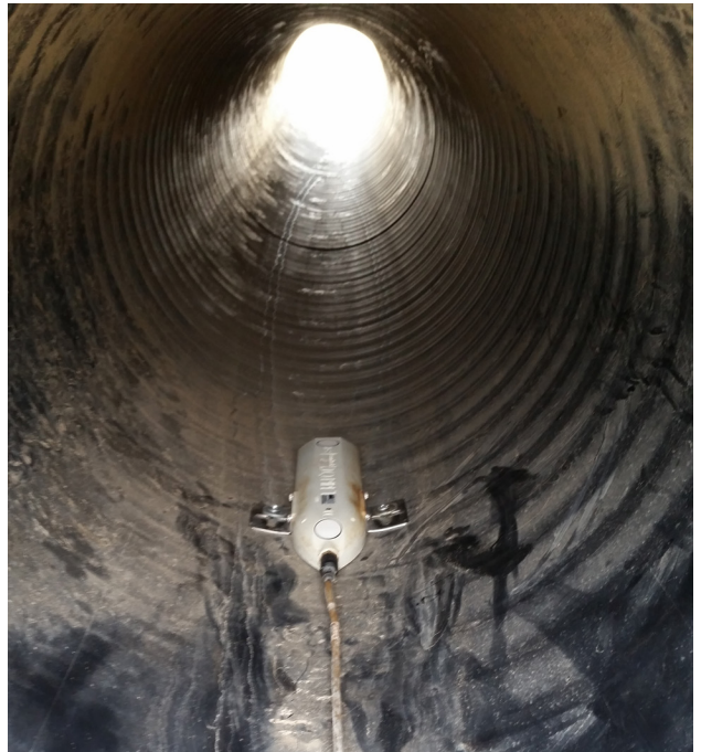
The SonTek-IQ Pipe is intended as either a bottom or top mounted flow meter that can be used in most industrial or agricultural applications. It can provide accurate flow values in pipes from 0.5m all the way to 5.0m, independent of whether these pipes are full or not.
